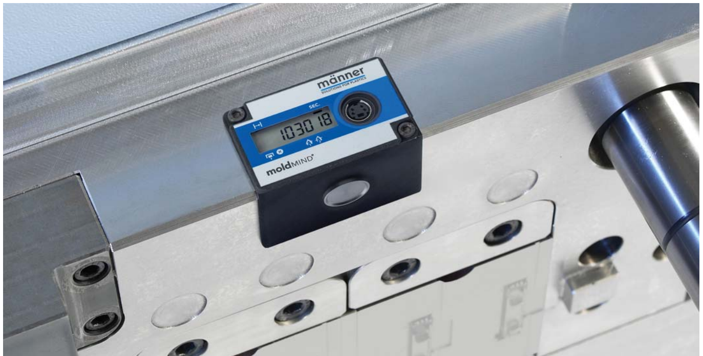
moldMIND®: "black box" for injection mold
