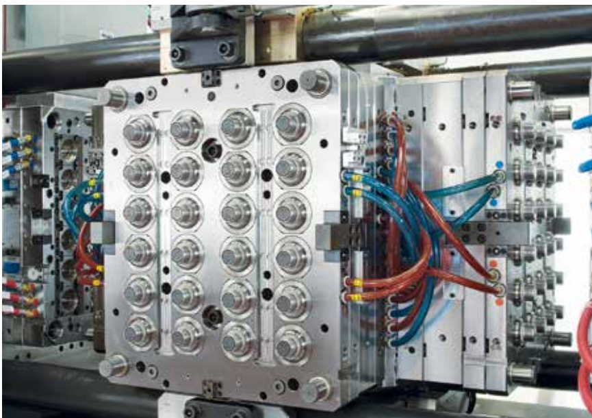
24+24-cavity cube mold of Foboha for the production of medical screw caps using 2-component technology (© Foboha)
